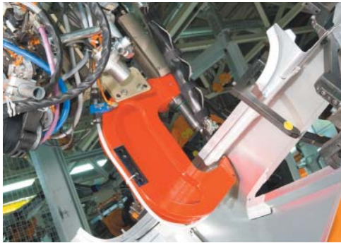
Solid punch riveting process in production
