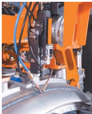
Laser welding process in production
